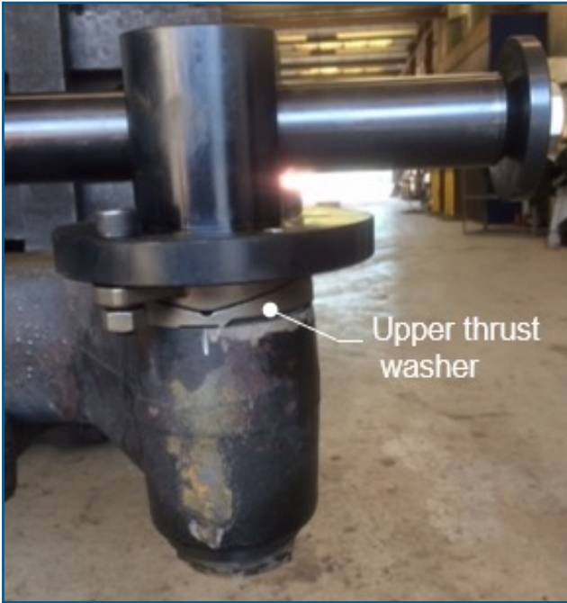
FIG 2. UPPER THRUST WASHER, FULLY SEATED READY FOR WELDING TO THE AXLE BEAM
